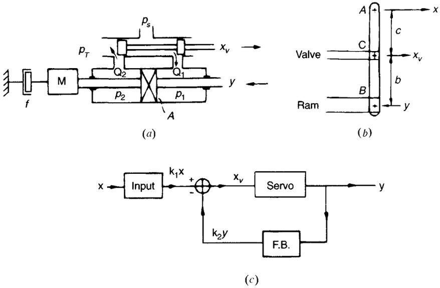
**Fig. 60.20** Simple open loop hydraulic servomechanism. (a) Open loop configuration; (b) feedback linkage; (c) closed loop block diagram.
