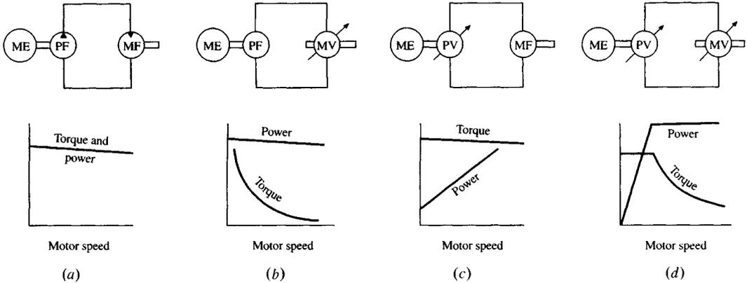
**Fig. 60.19** Pump and motor combinations. (a) Fixed displacement pump and fixed displacement motor; (b) variable displacement motor and fixed displacement pump; (c) variable displacement pump and fixed displacement motor; (d) variable displacement pump and variable displacement motor.
