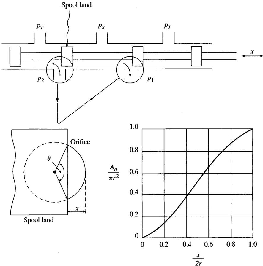
**Fig. 60.3** Effective exposed orifice area for a spool-type valve.
