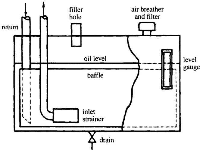
**Fig. 60.17** Pump set design. (a) The basic pump circuit; (b) layout of a typical hydraulic reservoir.
