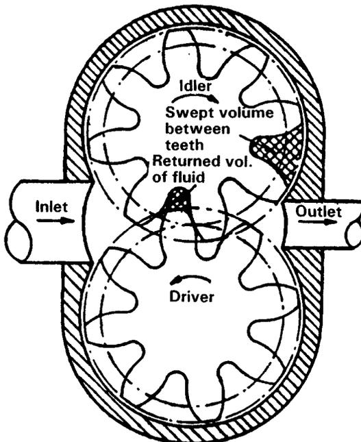
**Fig. 60.9** Gear pump construction.
