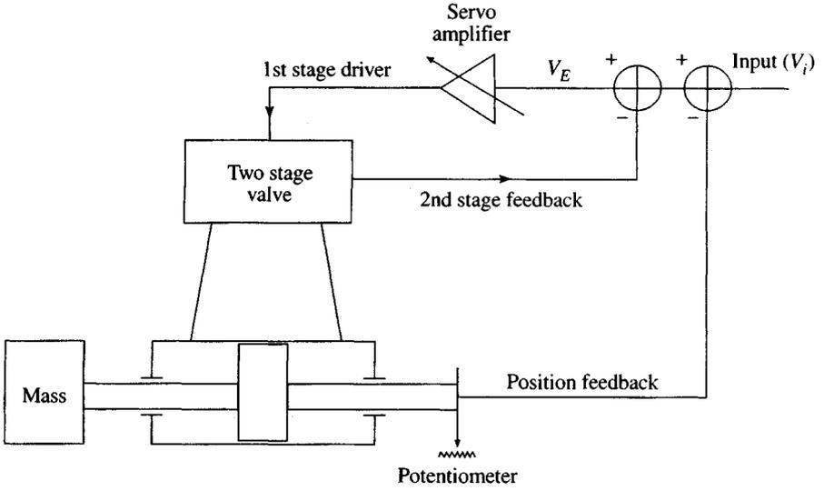
**Fig. 60.23** Two-stage valve–electrohydraulic servo system.
