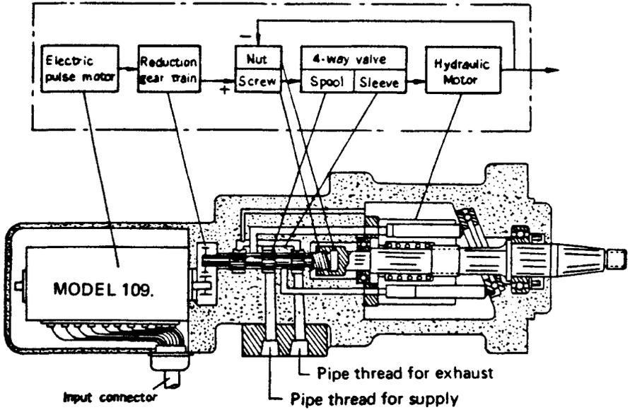
Fig. 60.26 Typical electrohydraulic stepping motor. (Courtesy of Fujitsu Ltd.)
