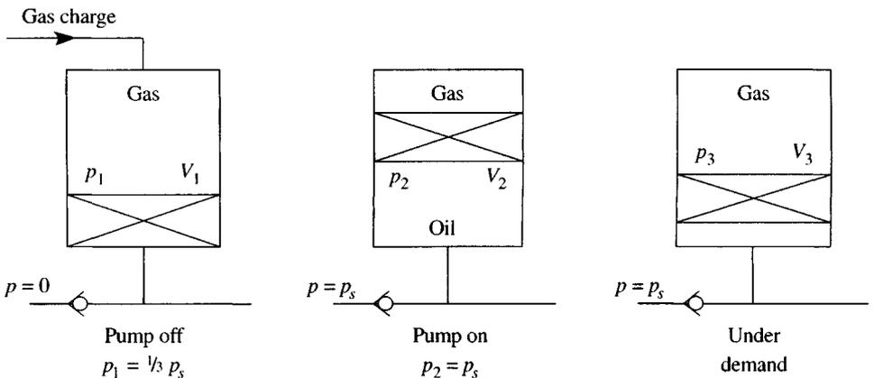
**Fig. 60.18** Accumulator operation.
