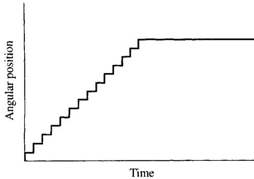
Fig. 60.28 Electrical stepping motor output.
