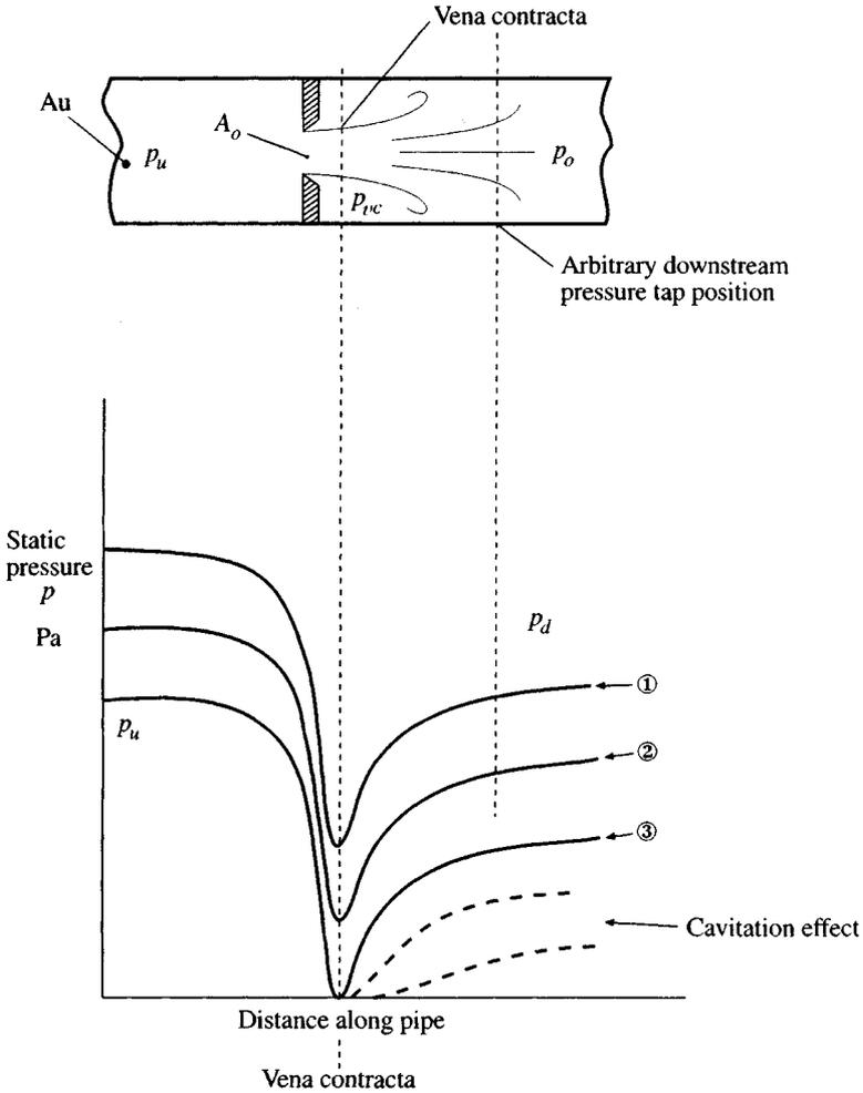
Fig. 60.2 Static pressure distribution.
