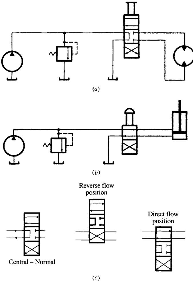
**Fig. 60.14** Simple hydraulic circuits and valve symbols. (a) Open-center valve control; (b) simple constant flow circuit; (c) valve symbol meanings.
