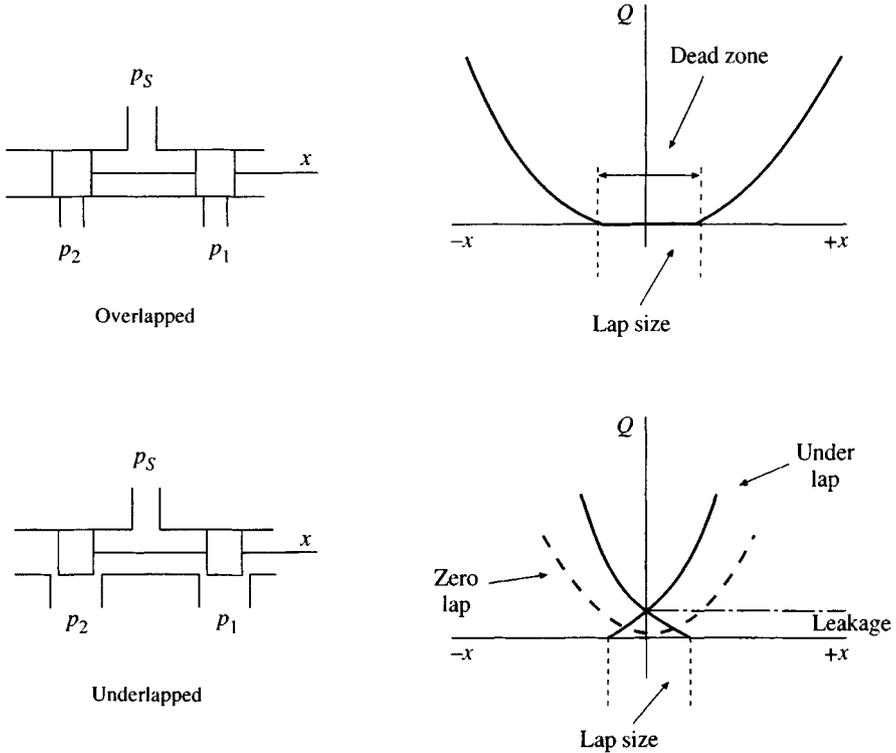
Fig. 60.4 Characteristics of valve lap.
