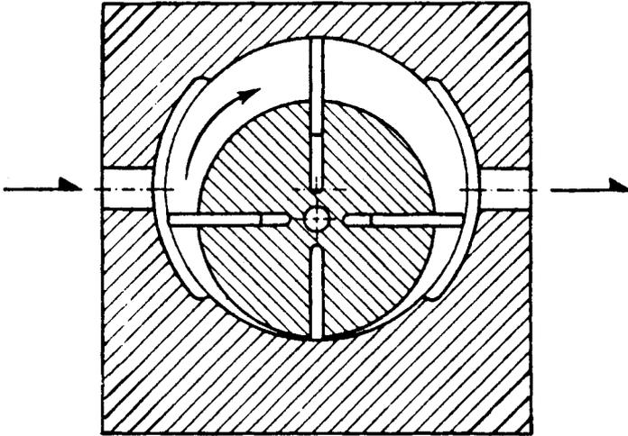
**Fig. 60.8** Schematic cross section through a vane pump. (From J. Thoma, *Modern Oil Hydraulic Engineering*. © 1970 Technical and Trade Press. Reprinted with permission.)
