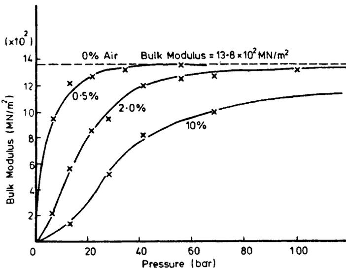
Fig. 60.12 Bulk modulus for a typical hydraulic oil including the effect of free air.
