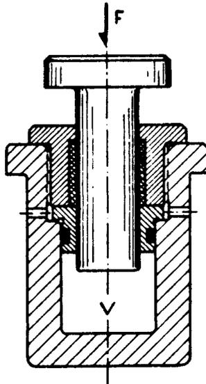
**Fig. 60.11** Pressure chamber for measuring compressibility. (From J. Thoma, *Modern Oil Hydraulic Engineering*. © 1970 Technical and Trade Press. Reprinted with permission.)
