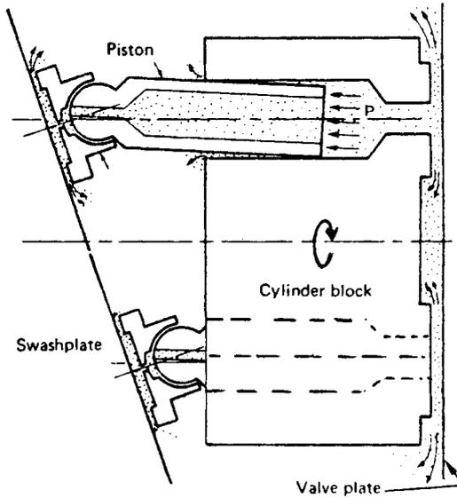
Fig. 60.1 Piston pump clearances.
