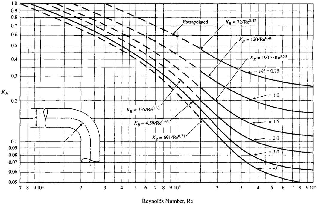
Fig. 60.6 Correction factor  $K_B$  for pressure loss in pipe bends.
