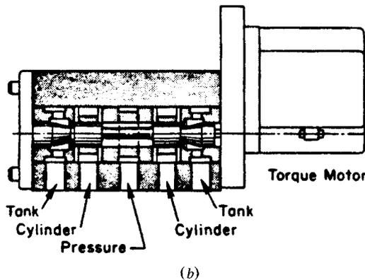
**Fig. 60.22** Typical electrohydraulic valves. (a) Two-stage valve (Moog Inc., East Aurora, NY); (b) single-stage valve.
