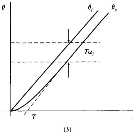
**Fig. 60.21** First order performance–time domain. (a) Step response; (b) ramp input;  $\theta = \omega t$  where  $t$  is time.
