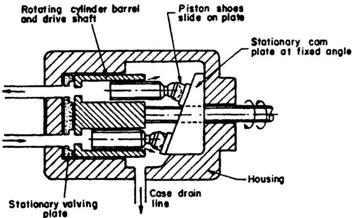
Fig. 60.7 Axial piston pump.
