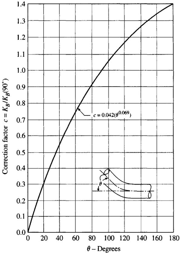
Fig. 60.5 Correction factor  $c$ . (Reproduced from AF Rocket Propulsion Lab., 1964.)
