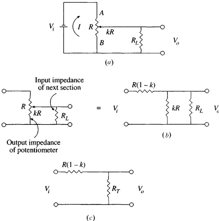
**Fig. 60.25** Potentiometer loading. (a) Actual circuit; (b) equivalent circuit; (c) least complex equivalent circuit.
