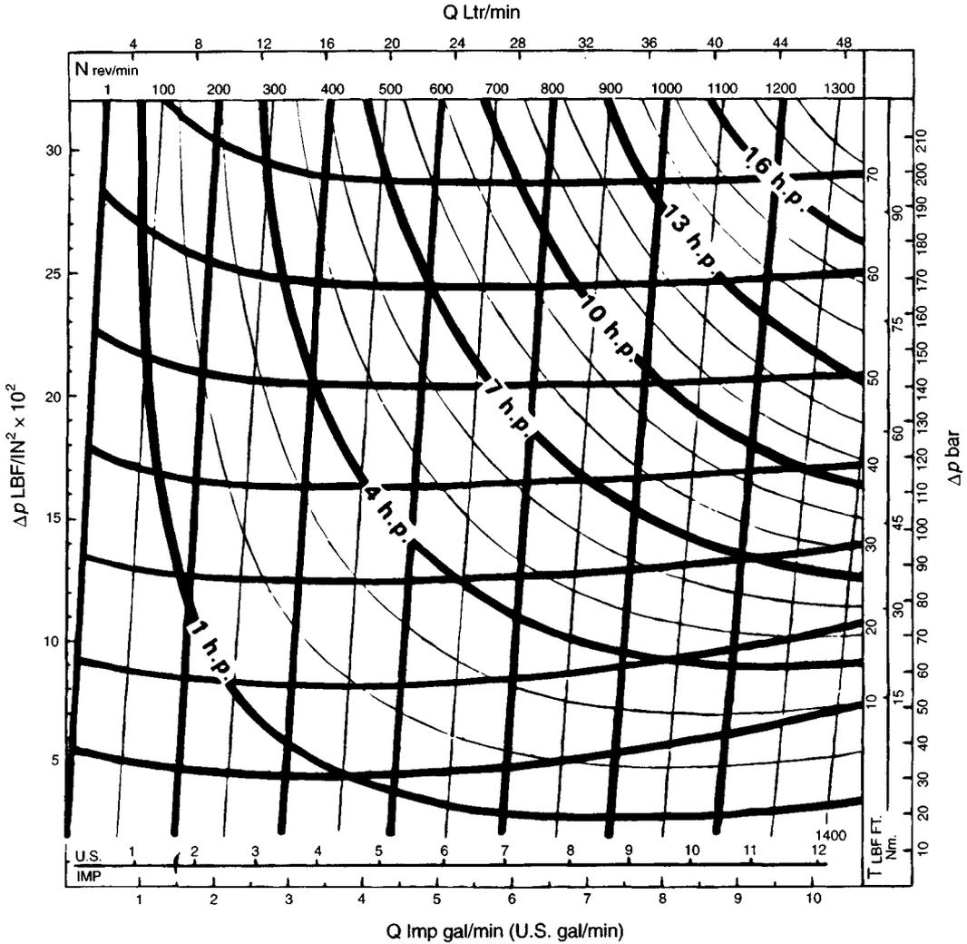
**Fig. 60.10** Typical performance range for a hydraulic motor, specifications appear in Table 60.6. (Courtesy of Kontak Manufacturing, Lincolnshire, England.)
