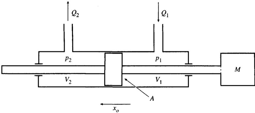
Fig. 60.13 Compressibility effects in a cylinder.
